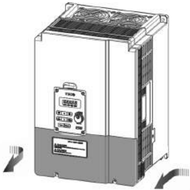
Step2: Remove the terminal cover
