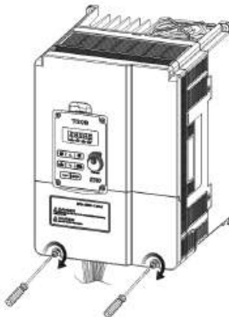
Step4: Tighten the screws
